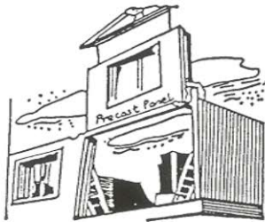
QUIC-SEAL 203 Applied Before Precast Panel Sits On It
