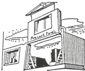
QUIC-SEAL 203 Applied Before Precast Panel Sits On It
